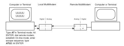
Figure 6-3. Digital Loopback Test (remote/automatic)
